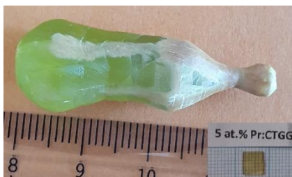
Figure 1: As-grown Pr:CTGG single crystal. The inset shows a polished crystal sample cut from the grown crystal.
