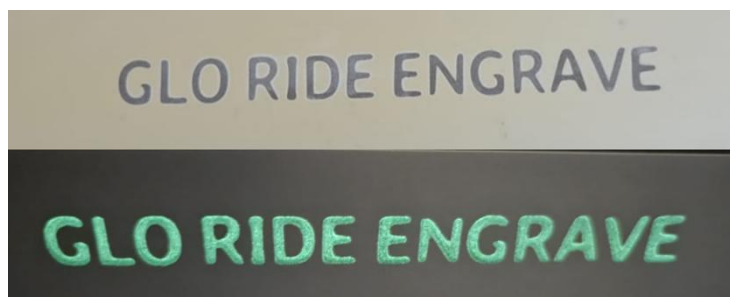
Figure 1: A persistent luminescent pattern embedded directly on aluminum surface.
